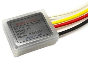
3<sup>rd</sup> Brake light flasher creates a brake light flashing effect to catch the attention of the drivers behind and avoid dangerous rear-end collisions. The flasher module is a microprocessor-based circuit specifically designed for brake light operations and packaged in a very tiny package. It works on both LED and incandescent bulbs. The flasher features a patented lockout time to minimize the brake flashing during the heaving traffic.
