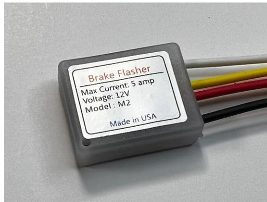
3<sup>rd</sup> Brake light flasher creates a brake light flashing effect to catch the attention of the drivers behind and avoid dangerous rear-end collisions. The flasher module is a microprocessor-based circuit specifically designed for brake light operations and packaged in a very tiny package. It works on both LED and incandescent bulbs.
