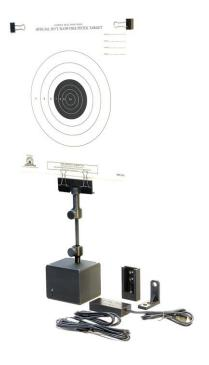
**Target Turner System (TTS) is** designed to assist with Bullseye and some ISSF disciplines' practice. The system is portable and can set at the range in minutes. The target turner box is mounted on a horizontal surface or tripod. Standard NRA style voice commands are given for Bullseye slow, timed, and rapid-fire courses. The 'attention' command is given for ISSF rapid (8, 6, and 4 sec) and 3/7 fire courses. The system is controlled by a smartphone or tablet.
